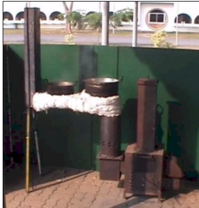
Figure 4: Gasifier stove under testing
