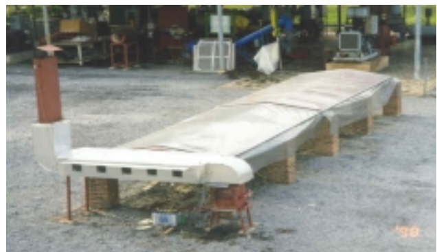
Figure 3: Solar-biomass hybrid dryer
